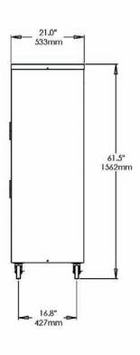
Minimum Wall Clearance Both Sides and Back -6 inches (152 mm)
