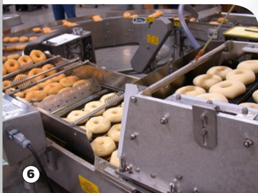
Above: 4– Standard Mark 6 system 5– Mark 6 system with automatic Proofer and Glazer 6– Automatic proofer with Deep Mark 6 fryer in Automatic system
